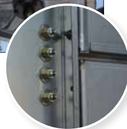
Extended Lubrication Lines with Grease Fittings Located by the Access Door
