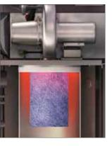
The modulating venturi premix burner and linkageless control automatically adjust the air/gas mixture for maximum efficiency and optimum turndown. A symmetrical, 360° even-temperature heat output is achieved from the burner, providing clean combustion with ultra-low NOx emissions of less than 20 ppm as standard and less than 9 ppm as optional.
